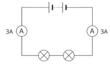
The **current is the same** everywhere in a series circuit. It doesn't matter where you put the ammeter, it will always show the same reading. The more cells or batteries you add, the greater the current. Current is **not** used up.
