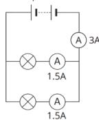
The **current is split** between the branches in a parallel circuit.
